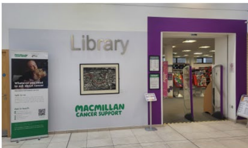
New and clearer signage at zones within the centre such as the library. Contrasting colour to make entrance clearer, coloured strips on entrance/exit barriers for sight impaired individuals.
